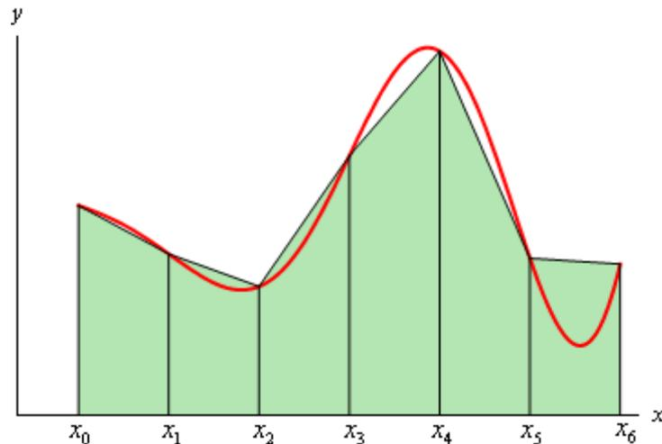
Figure 1: Illustration of the trapezoidal rule
